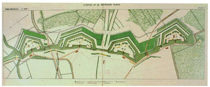
Fort near Jutphaas and Fort Vreeswijk. The first series of forts on the Waterline were simple structures, consisting of earth ramparts, located at the centre of the road or quay to be protected. The forts were surrounded by a moat and the gun emplacement was on the main rampart. The shape and size of the forts were dictated by the width of the access and the location of the constructions that enable inundation. Apart from the Lunettes, the forts did not yet have stone buildings.
